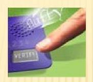
Beepcard, a company in California, has designed a credit card that works only when it recognizes the voice of its rightful owner. Enclosed in the card is a tiny microphone, a loudspeaker and a speech recognition chip that compares the spoken password with a recorded sample. If the voices match, the card emits a set of beeps that authorize a transaction over the telephone or the Internet. If the voices do not match, the card will not beep.
